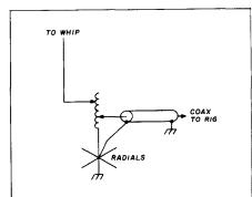
fig. 7. Single coil resonates whip to 3/4-wave mode and also permits match to coaxial line. For 14 MHz, coil is 12 turns of No. 12 wire, spaced twice wire diameter, wound on a ceramic form 2 inches in diameter. Adjust taps for best match as described in text.
